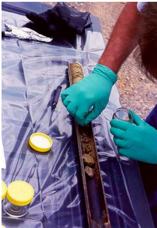
Pictured is a split spoon sampler being used on the Greenway Chemical Project site by LD&A Senior Technician Conrad Majors.
